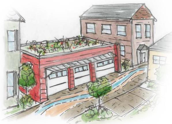
**7 Green roof** - Add where possible on flatter rooftops. Waterproof roof membrane with lightweight soil medium and plants. Soil and plants absorb water, preventing runoff to the street or sewer system.
